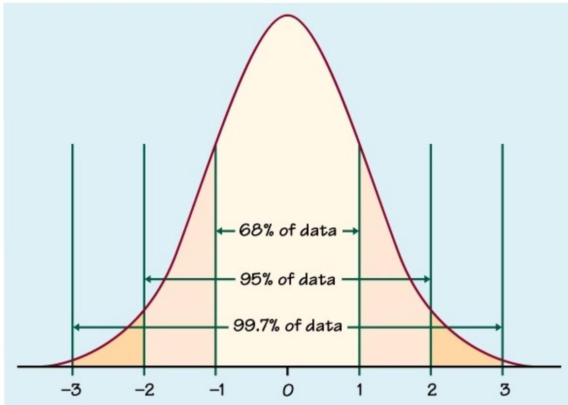
Area under the Gaussian distribution curve
